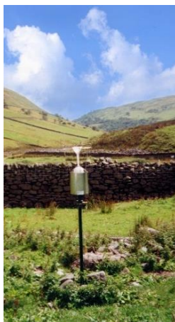
Figure 4 Bulk rain sampler (Bannisdale)
